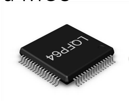
LQFP (Low-Profile Quad Flat Package)
