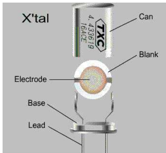
(Fig.7) (a) Metal can type resonator (b) Ceramic SMD type resonator (c) Symbol of crystal unit
